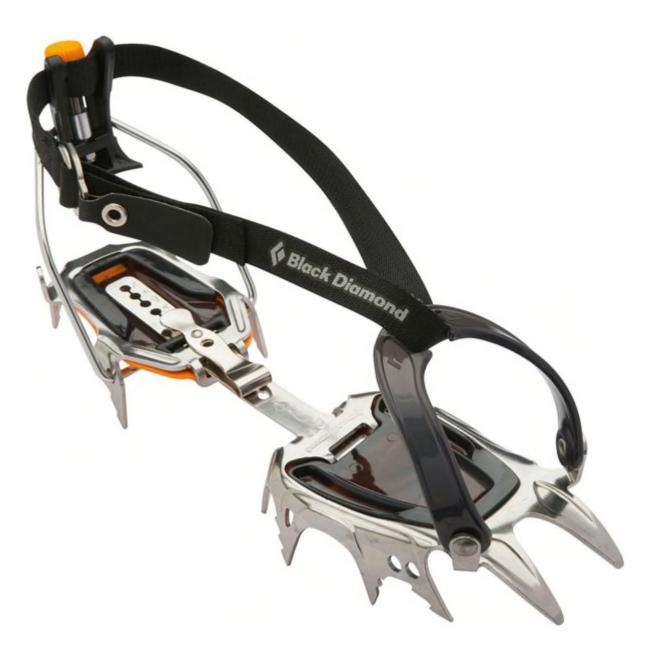
C3 crampons have a metal bar at the front and are typically used for technical climbing like ice and mixed climbing. They are only compatible with a B3 boot that has a toe welt. Suitable trips: Mont Blanc, Monte Rosa, Ice Climbing
